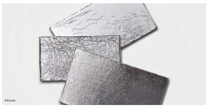
Vacuum insulation panels (VIP): A support core made from compressed silica powder is shrink-wrapped in a multi-layer special film. Insulation panels filled with fumed silica provide excellent insulation against heat and cold.
